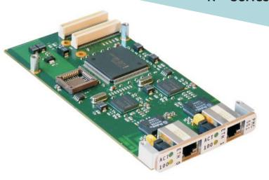
on-board Intel® 82551 controllers manage the Ethernet protocol (including checksums), thereby alleviating the processing load of the host CPU.
