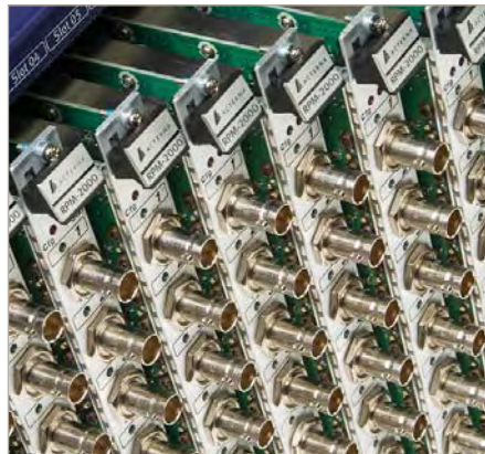
Close-up view of the rear of a HCU1500 showing RPM2000 modules.
